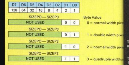
Fig. 1: Bit assignments for size registers SIZEPO — SIZEP3. (53256 — 53259)
